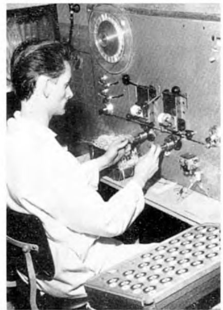
The cutting machine senses a cutting signal recorded on the tape and stops in precisely the correct position for the operator to cut. Complete programme copies, together with leaders and hubs, are placed on the tray on the right
