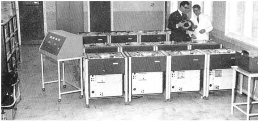
The copying room at Walthamstow. The first bank of four machines are the two pairs of "mothers"; the eight "slaves" can be seen behind them. Ron Holmes, Works Manager, left, is talking to one of his technicians
