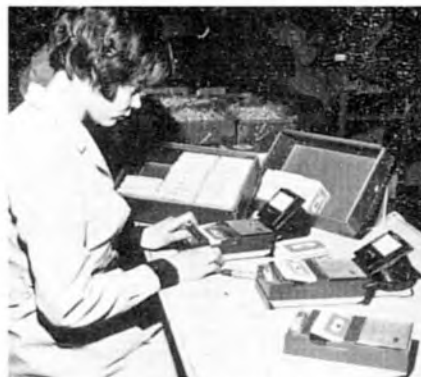
Each Musicassette is tested at the beginning and end of its programme. Note the apparently standard playback machines used for this task. The meters attached are simply to keep a check on current consumption, which must be within certain fixed limits
